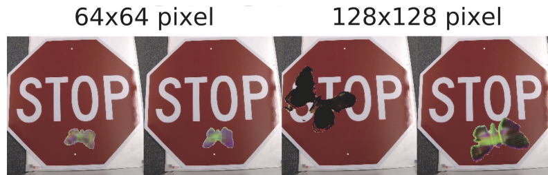
Figure 5: Moth-like patches on a STOP sign can make autonomous driving cars misrecognize it as Speed Limit 80 [342].
